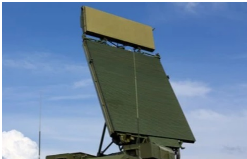
Figura 14 – Antena Phased Array .
