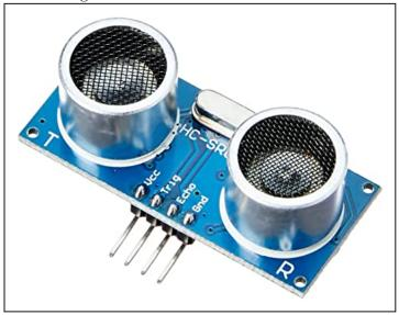
Figura 18 – Modelo do sensor HC-sr04
