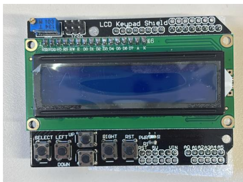
Figura 11 – Display LCD 16X2 Shield
