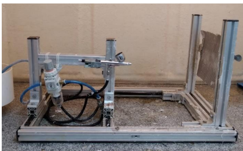
Figure 7 – Photograph of the experimental setup used for the solution blow spinning (SBS) process
