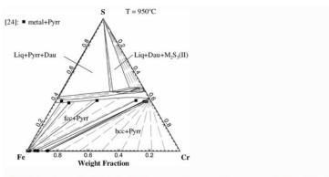
Calculated isothermal section of the Cr-Fe-S phase diagram at 1223.15 K (950 °C) together with experimental data; experimental tie-lines shown as solid lines; calculated tie-lines shown as dashed lines; Abbreviations: bcc stands for the body-centered-cubic Cr-Fe-alloy phase, fcc for the face-centered-cubic Cr-Fe-alloy phase, Dau for Daubréelite and Pyrr for Cr-Fe-pyrrhotite
