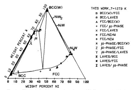
Fig. 1—The optimized isothermal section at 1273 K compared with the experimental data obtained in the present work. Lambda  $(\lambda)$  is used to denote the Laves phase.
