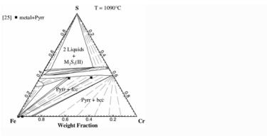
Calculated isothermal section of the Cr-Fe-S phase diagram at 1363.15 K (1090 °C) together with experimental data; experimental tie-lines shown as solid lines; calculated tie-lines shown as dashed lines; Abbreviations: bcc stands for the body-centered-cubic Cr-Fe-alloy phase, fcc for the face-centered-cubic Cr-Fe-alloy phase, and Pyrr for Cr-Fe-pyrrhotite
