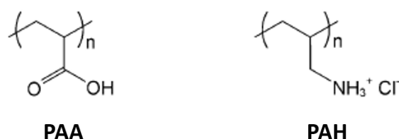
Figure 2.9: Repetition unit of PAA and PAH polyelectrolytes [194]
